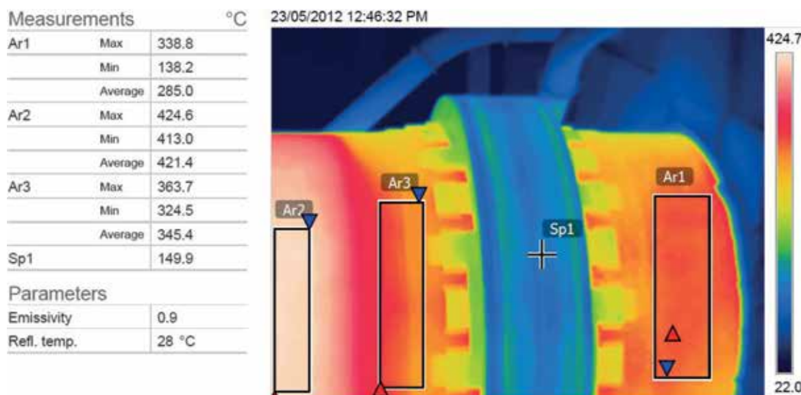
Figure 15: Infrared Thermography picture of burning zone – 13mm ISOMAG Insulation Photo taken: May 2012 (E60 FLIR Camera – M Taddeo)
