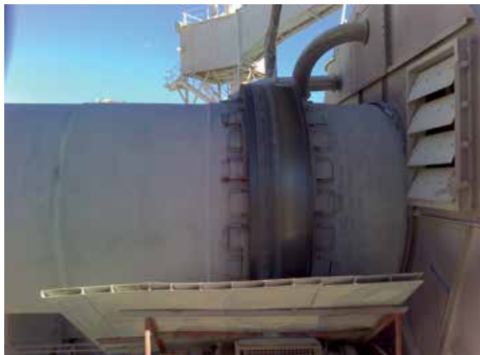
Figure 3: No.1 Tyre in Burning Zone of BC Marulan No.2 Kiln
