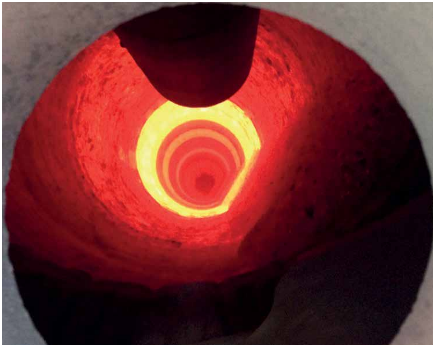
Figure 26: Insulated Brick lining comparison 20 minutes after flame out Photo taken: 16 January 2014 (Boral Cement Marulan Sth)
