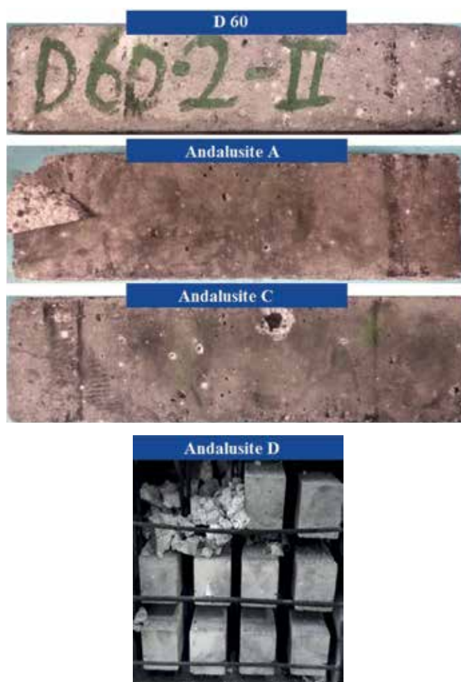
Fig. 3: Castable prisms after CO resistance test (ASTM C288) 200h at 500°C
