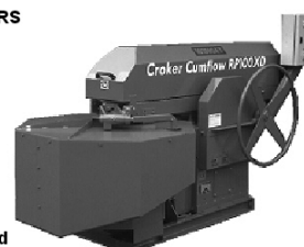
CROKER CUMFLOW RP100XD MK2 (113 litres, 163kg capacity)
