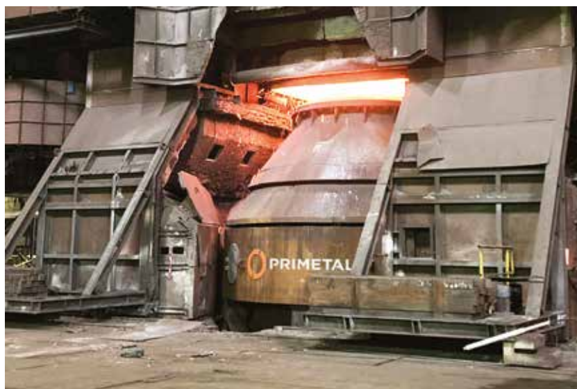
The new 125-ton LD converter (BOF) at ArcelorMittal Zenica's steel plant ensures increased productivity and has eliminated a sloping issue
