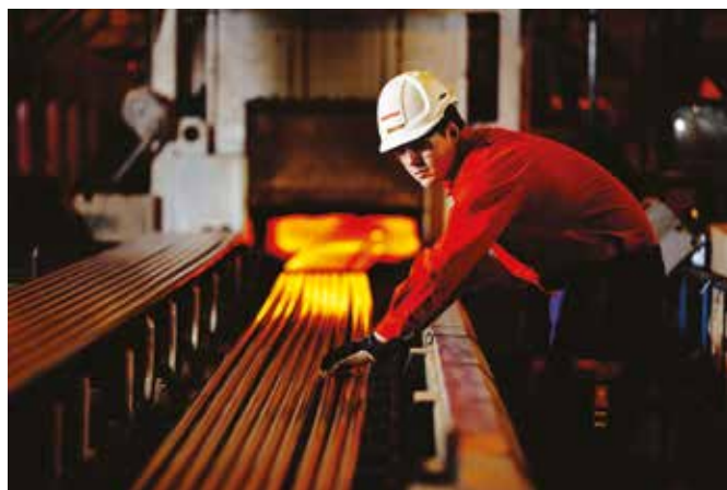
Roller hearth is one furnace type in steel manufacturing that can be electrified to reduce CO 2 emissions
