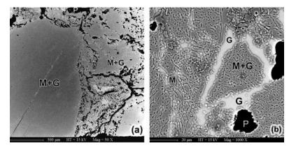
G = Glassy Phase formed on sintering A high temperature glass softens.
