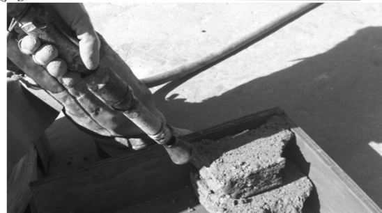
Hand-held pneumatic rammer is used to consolidate the refractory
