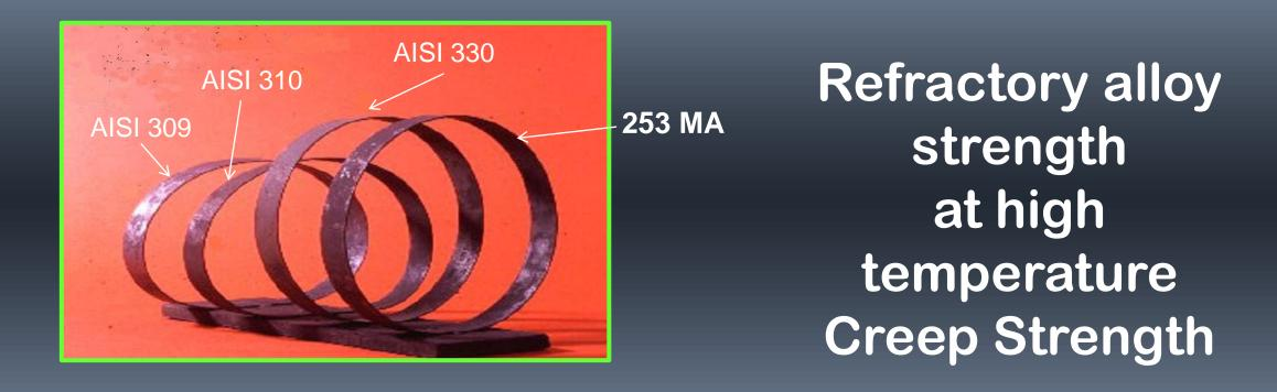
35 hours at 1000° C for alloy rings having a thickness of 1 mm AISI 310 and AISI 309 deformed under their own weight (Creep Deformation)
