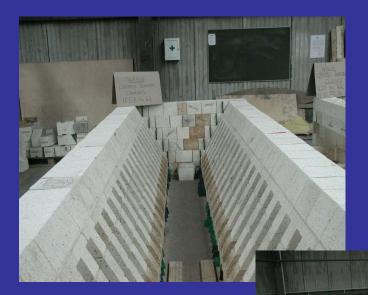
A ceramic burner for a hot blast stove designed to allow gas mixing through the burner slots
