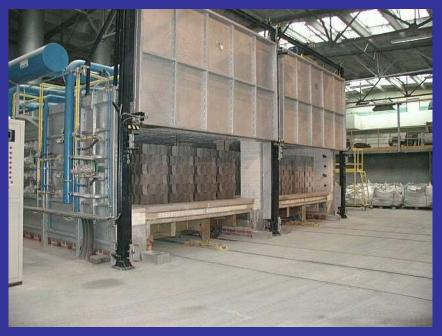
Drying is the first operation in the tempering process and is critical. In some cases the drying process is undertaken in the entry part of the tunnel kiln where low temperatures and humidity can be controlled. Bricks are dried according to their shape and size to avoid undue stresses which can generate or develop faults in the subsequent firing process.
