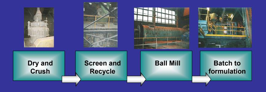
Raw materials are processed by drying, crushing, screening and milling to produce a wide range of size fractions from millimetre to micron sizes. Air swept ball mills produce the very fine flour grades. High purity materials are pre-processed and pre-blends may be purchased.
