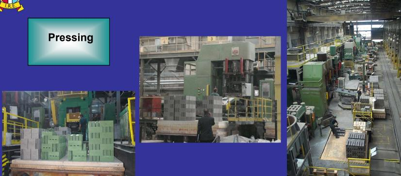
Most bricks are machine pressed.
