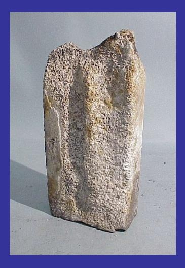
A bricks after service in a Chlorinator where chlorine gas has reacted with the alumina content of the brick and left a weakened and friable surface
