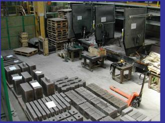
Some bricks are not able to be machine pressed. This is most commonly because of shape complexity but low quantity items may follow this route to avoid the high cost of press moulds. Pneumatic rammers are used on mixes formulated for hand forming. The technique of hand moulding is an acquired skill and there are procedures to be followed to ensure a high quality product. Controlled drying is applied to bulky shapes. It is also possible to cast and fire special shapes.
