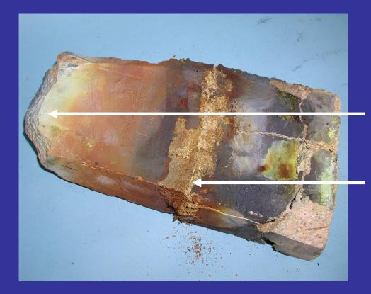
Another brick after service in a Chlorinator where chlorine gas has reacted with the alumina content of the brick and left a weakened and friable surface
