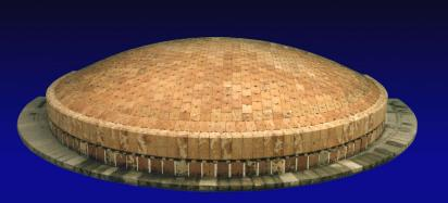
**Pre-assembly of a full furnace roof**
