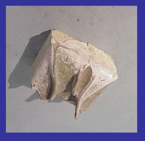
A silica brick from the roof of a glass furnace.
