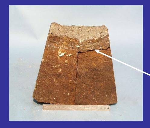
Basic bricks from a combustion chamber.
