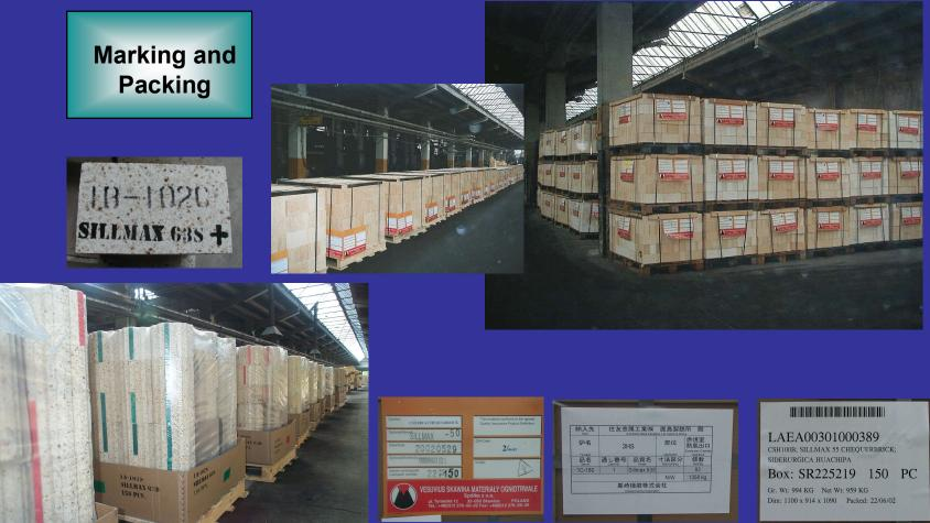
The final stage of the operation is the marking/labelling of the bricks and the appropriate packing for transit to the final destination. Bricks may be individually marked or colour coded. Pallets may have special packaging and/or labelling. Traceability codes form part of the labelling
