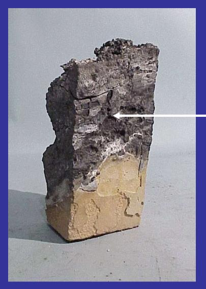
A bricks that has been in molten aluminium. Corundum (alumina) is growing inside the brick texture and densifying the brick texture.
