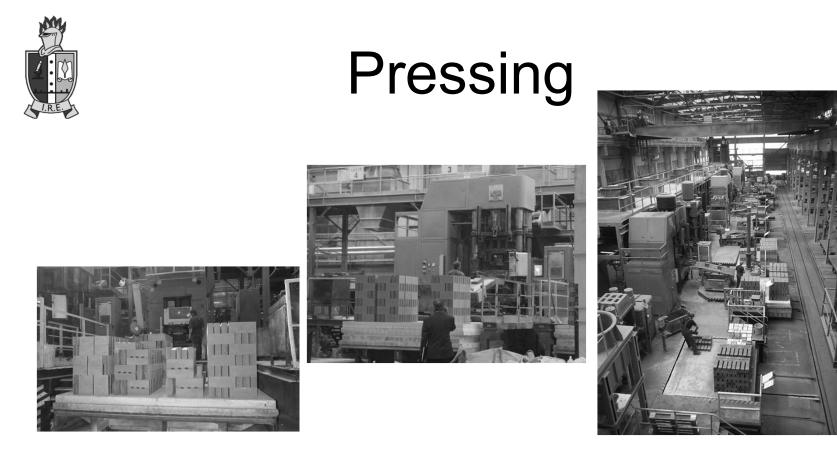
Most bricks are machine pressed.
