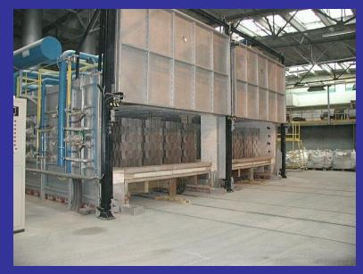
Drying is the first operation in the tempering process and is critical. In some cases the drying process is undertaken in the entry part of the tunnel kiln where low temperatures and humidity can be controlled. Bricks are dried according to their shape and size to avoid undue stresses which can generate or develop faults in the subsequent firing process.
