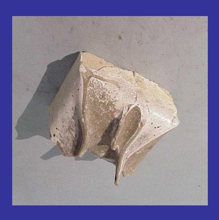
A silica brick from the roof of a glass furnace.
