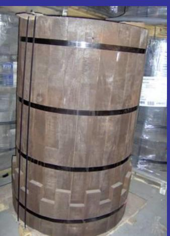
A preassembled snorkel for a steelmaking RH vacuum degasser.
