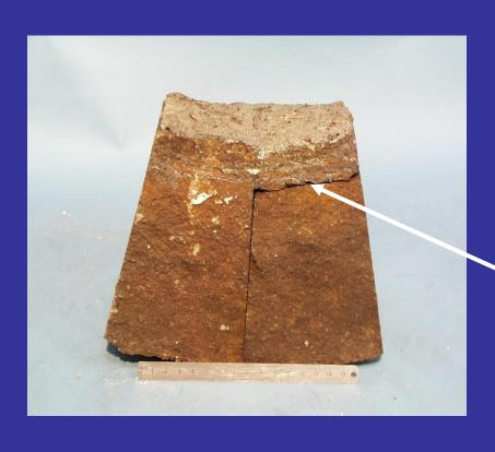
Basic bricks from a combustion chamber.
