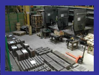
Some bricks are not able to be machine pressed. This is most commonly because of shape complexity but low quantity items may follow this route to avoid the high cost of press moulds.
