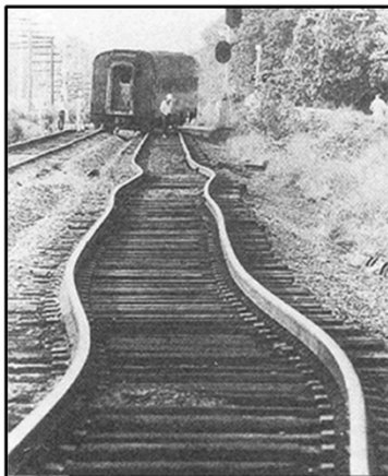
Thermal Expansion of railroad track due to excessive heating. Yes, they would close the track at this point! (Notice the derailed car in the background.)
