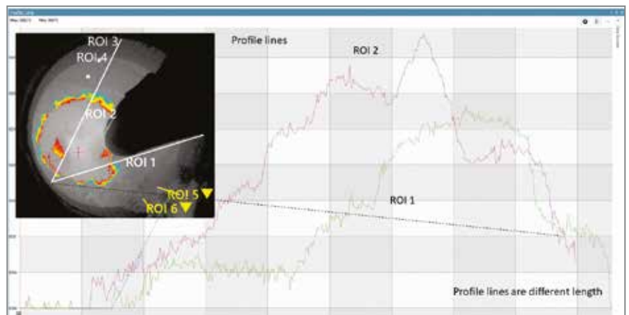
Fig.2 Rotary cement kiln with isotherms and thermal profile lines
