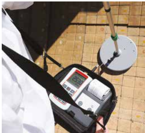
The device uses electromagnetic measuring through the eddy currents principle to determine brick thickness. The magnetic probe is placed against the brick, and the 4-digit display shows the measurement in centimetres
