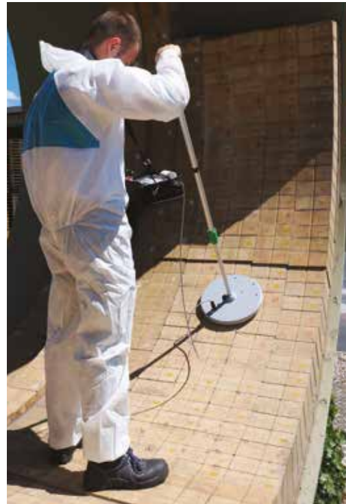
The handheld instrument measures and displays the thickness of refractory brick and concrete for industrial ovens, kilns and furnaces as well as unreinforced refractory concrete
